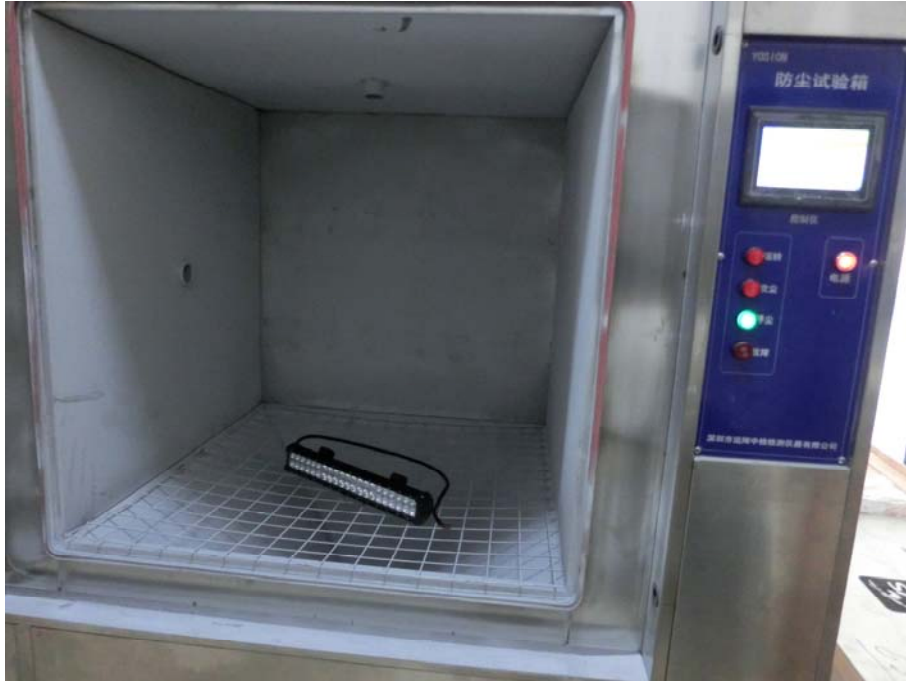
Photo 1 IP 6X test Over View
