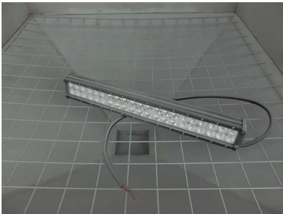
Photo 2 After IP 6X test Over View
